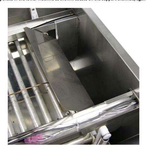
Loosen the nuts holding on the cam shaft brackets and slip the stacking chute lock under the nuts and lock washers. Slide the stacking chute lock tight against the stacking chute and tighten the nuts.
