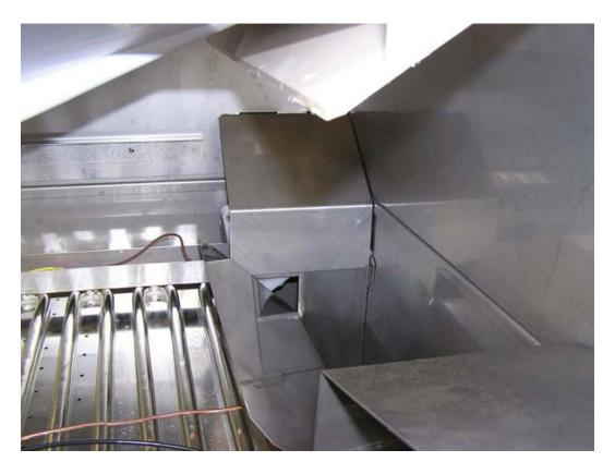
Remove the bin probe of the upper machine from the bin probe holder by gently tugging on the wire after removing the tape. Feed the bare bin probe through the hole in the bottom of the top machine's floor then the grommet and finally insert the bin probe in the bin probe holder and install into a pre-cut hole next to the bottom machine's bin probe.
